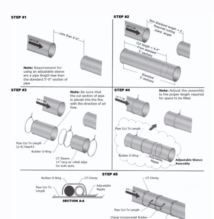
O-Ring and Rolled End from the Adjustable Sleeve for sealing purposes
